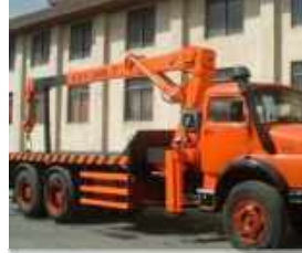
Truck mounted crane 10 tons
